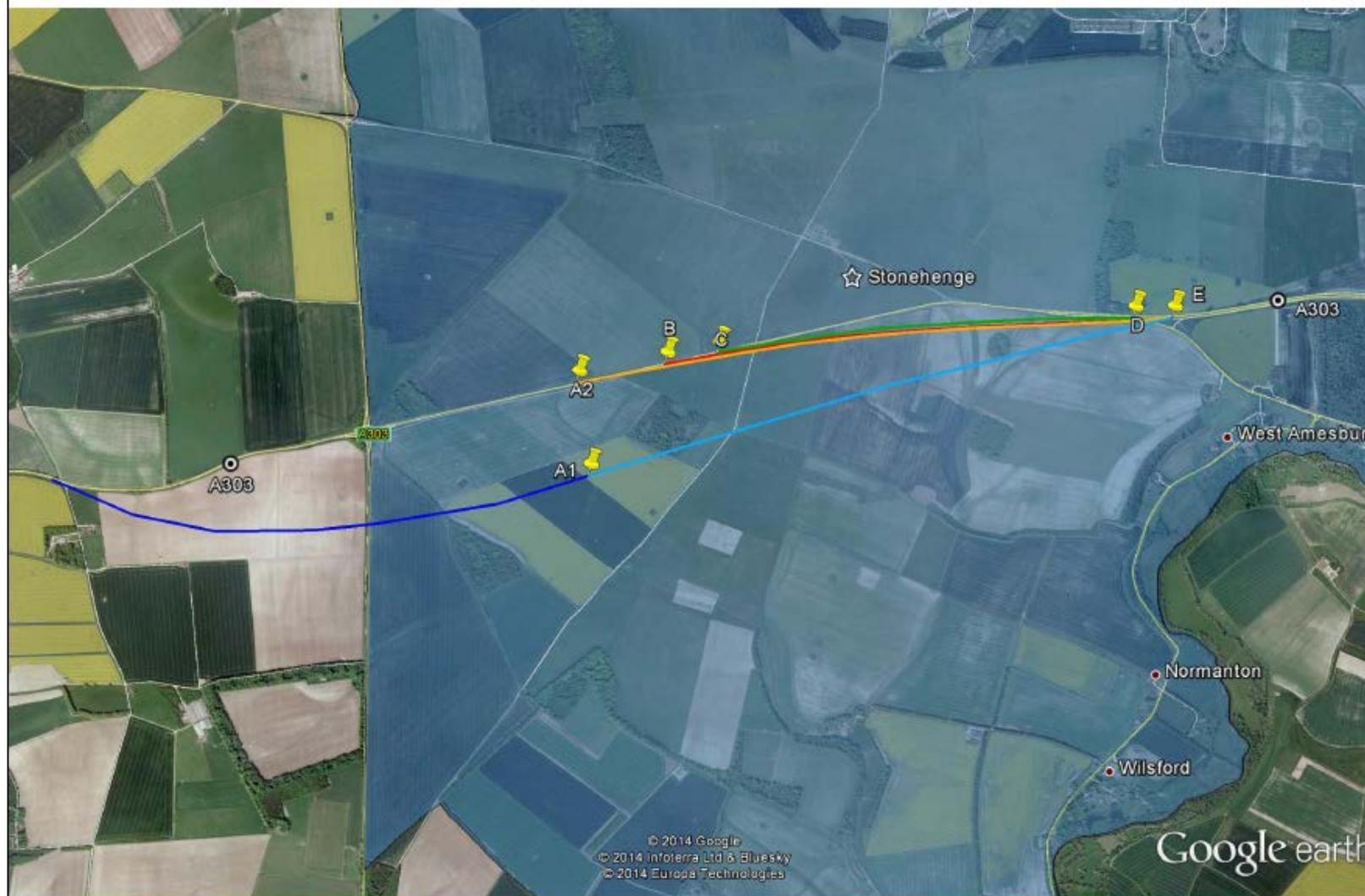
**Fig 3** locations of tunnel portals for 2.1km published scheme (Portal C & D), 2.5km on-line tunnel (Portals E & B), 2.9km on-line tunnel (Portal E & A2), 2.9km off-line tunnel (Portal E & A1) (Tata 2014, Appendix B, 1)
